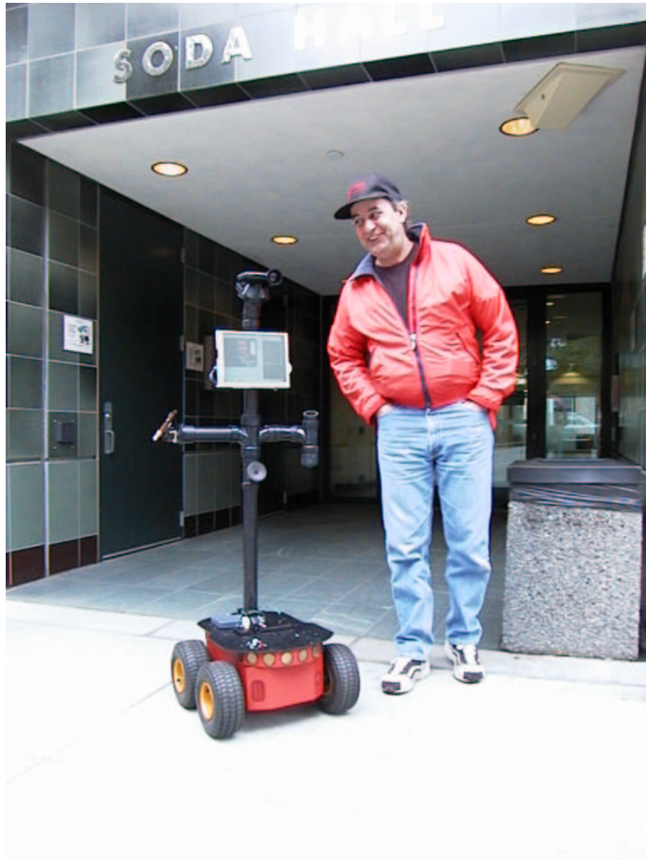
Figure 9.3: PRoP 1 during Experiment 2 as operated outside the computer science building at UC Berkeley. The remote user is controlling the PRoP from Denmark in this image.
