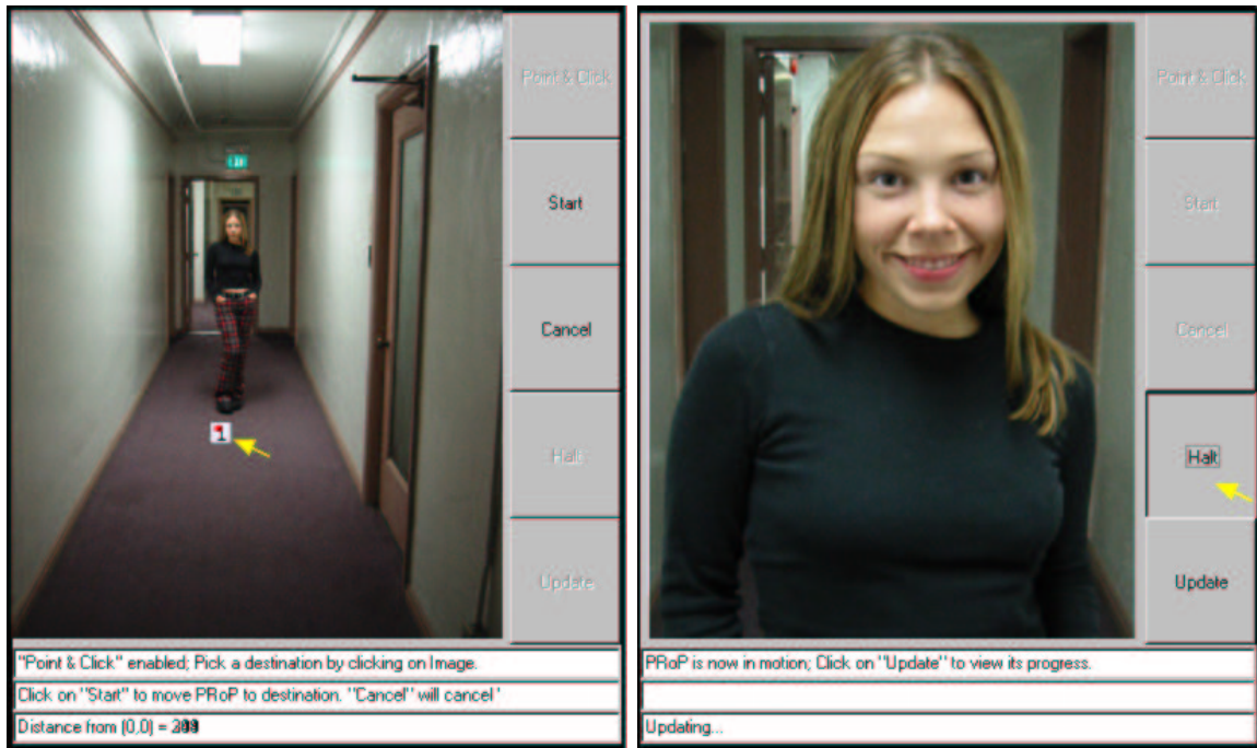
Figure 11.1: Two views of the prototype point and click interface. Before selection (left) and after completed motion (right).
