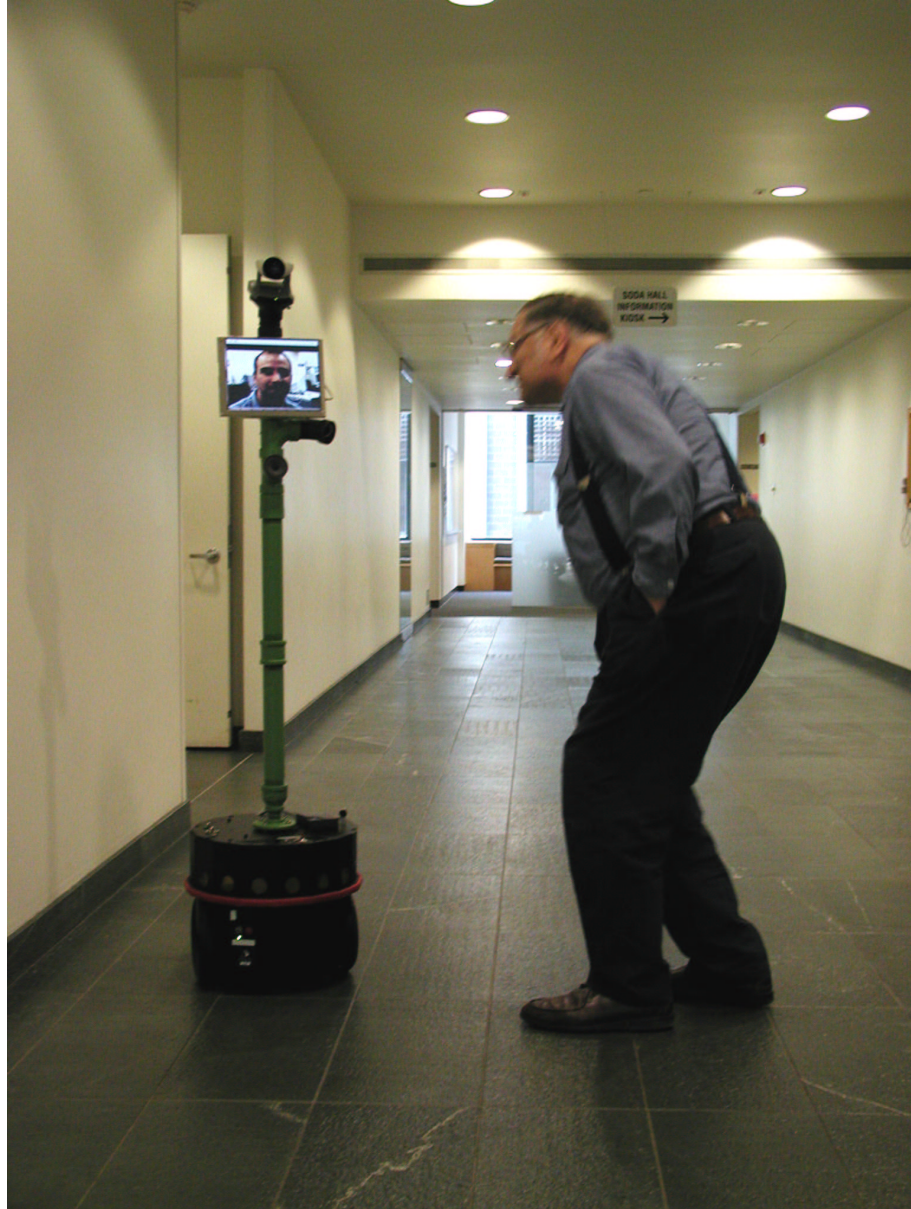
Figure 7.11: An encounter with PRoP 2. Notice the locally embodied participant focusing his gaze cue onto the screen rather than the camera. This is a common issue with any form of video-conferencing.
