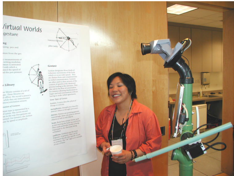
Figure 7.12: From a remote location a primary user interacts and discusses the contents of a poster with a secondary user though PRoP2 .
