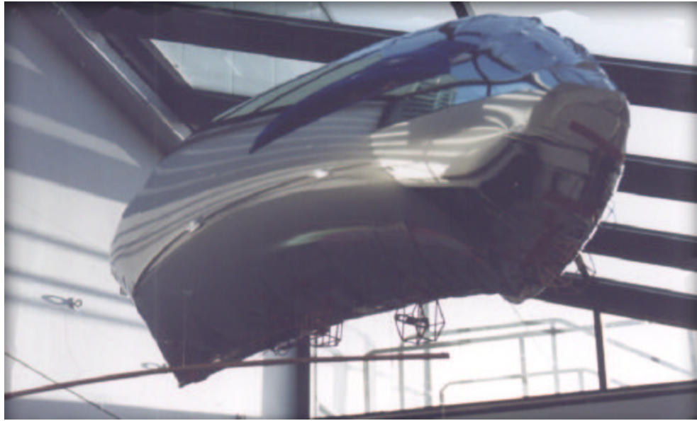
Figure 6.7: One of the smallest space browsing blimps designed at just under a meter in length. Using Mylar greatly decreased the blimp size but radically increased its fragility. Impressive blimps with short lives.
