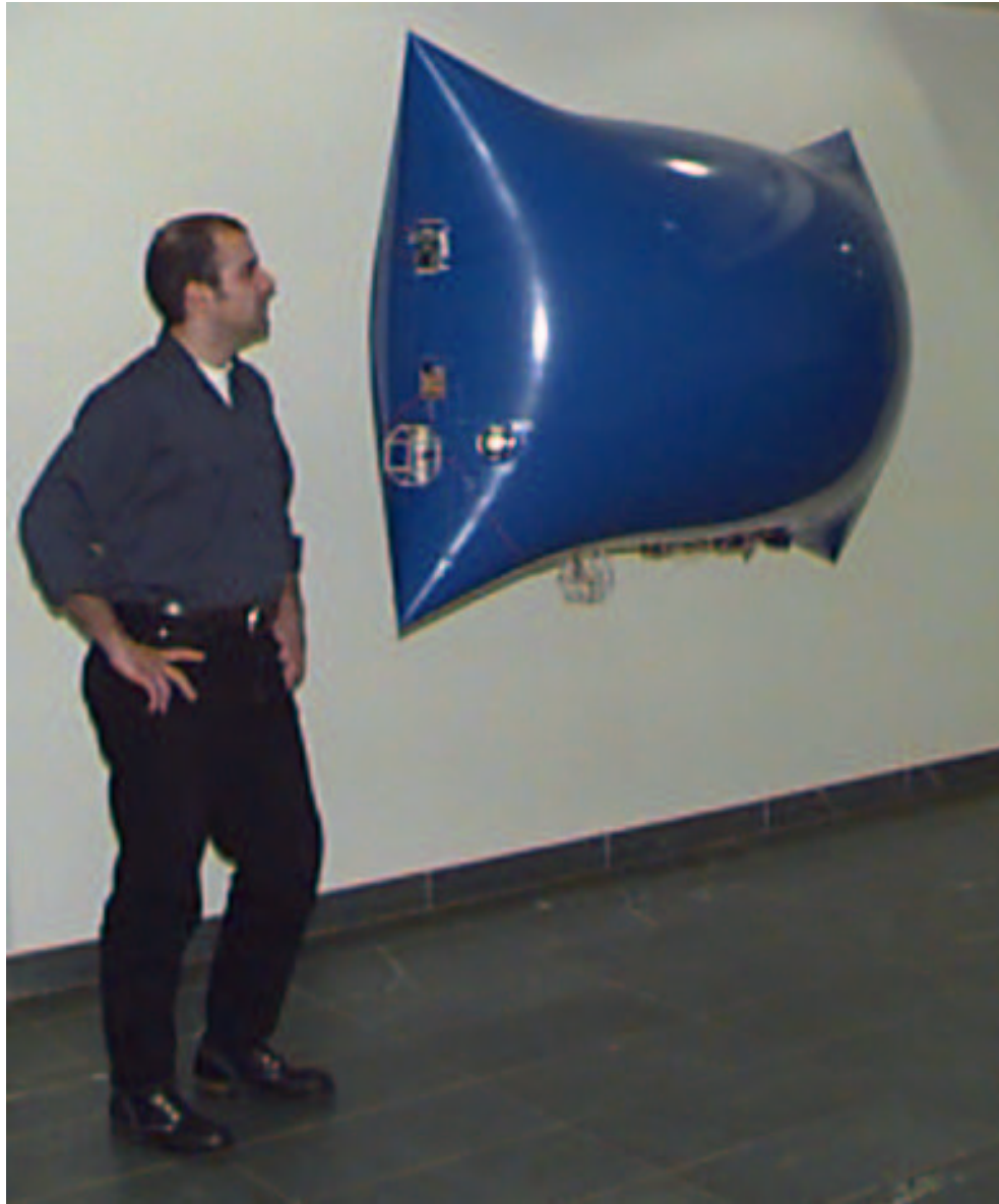
Figure 6.4: An medium-sized blue polyurethane space browsing blimp interacting with a person.
