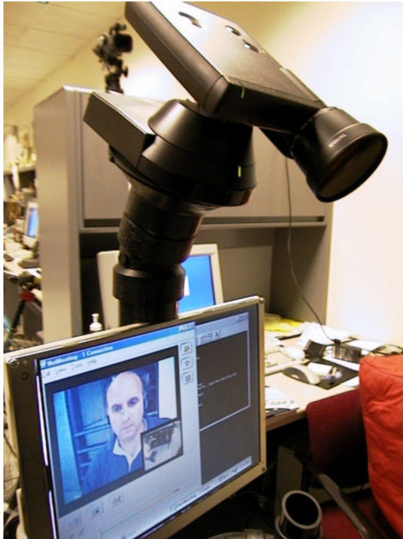
Figure 9.4: Close-up view of PROP 1 during Experiment 2 while under the control of a remote user in Denmark. You can see his video image on the screen while the inset image is the view he is receiving.”
