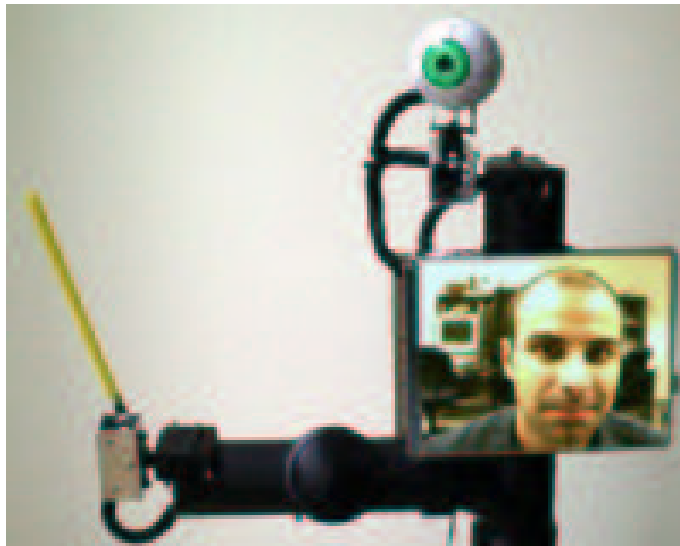
Figure 7.4: A view of the hand/arm pointer, eyeball camera head, and display screen on PRoP 0.
