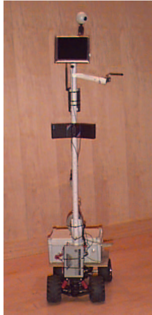
Figure 7.2: One of the earliest PRoP prototype systems. A modified remote control car base with attached hardware (circa 1996).
